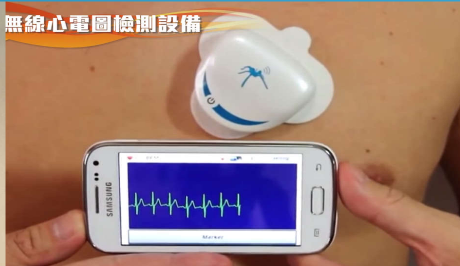
Wireless iOS bluetooth ECG machine
